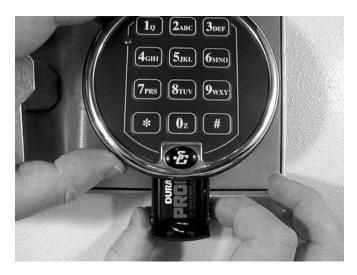
4. With the new battery in the holder, slide the holder into the base of the keypad until it clicks into place. If your lock does not operate properly, don't press any buttons for five minutes, then try it again.
