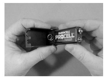
2. As you remove the old battery, you will notice there is a spring at the bottom of the holder. The new battery will rest on top of this spring to maintain good electrical contact.
