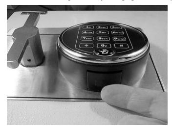
1. Keypad disassembly is neither required nor advised. The removable battery holder is accessed from the bottom of the keypad base. Pull it slightly toward the front of the keypad, then downward to remove it.
